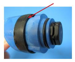
Replace the battery cap gaskets with the provided gaskets and lubricate the indicated surface with the lubricant provided.
